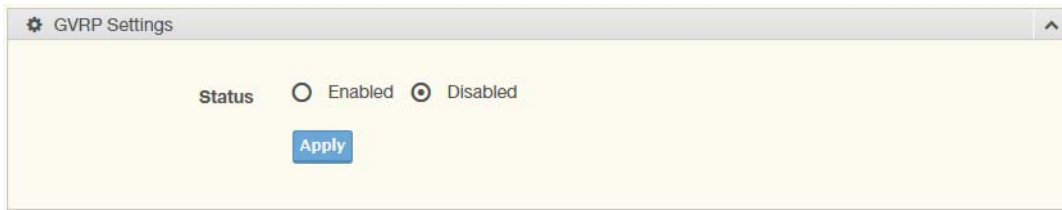
Figure 4.30 L2 Switching > GARP > GVRP Settings
