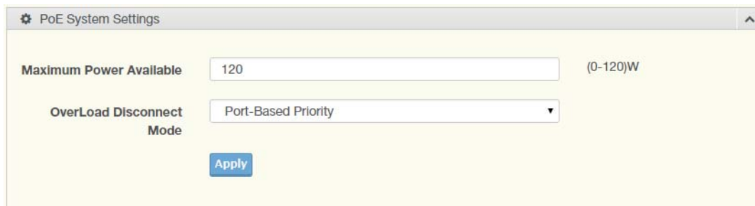
Figure 4.113 Management > Power Over Ethernet > PoE System Settings
